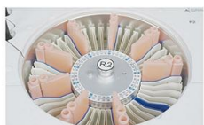
Reagent Tray 2~8°C cooling for 24 hours.
